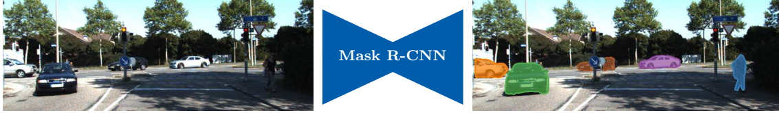
Figure 4.2: The set of rigid bodies \mathcal{O} is defined as the set of objects detected by an instance segmentation (colored in the right image) and the background.
