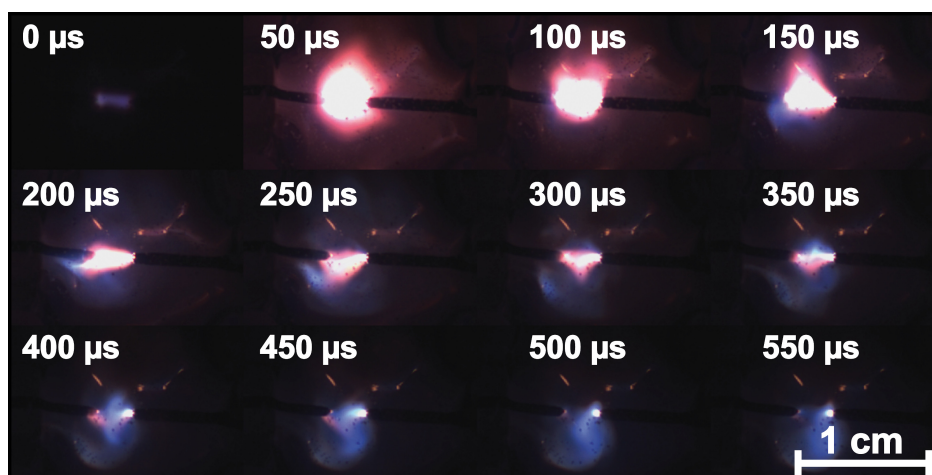
Figure 4.3: High-speed photographs of an arc discharge where the capacitors were charged to 450 V. Picture one (0 \mu\text{s} ) shows the weak ignition spark.
