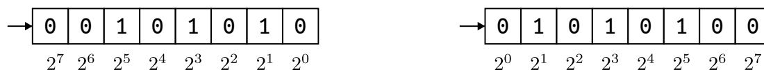
Figure 3.5: Bit order of unsigned integer numbers on different architectures. The memory pointer is illustrated by an arrow pointing to the first bit that is read. Left: big-endian, i.e., the first bit accessed is the one corresponding to the largest value. Right: little-endian, the least significant bit is stored in the first position. The difference is irrelevant for usual integer and floating-point arithmetic. However, using algorithms that operate on the integers' bits directly requires awareness of the system's architecture.
