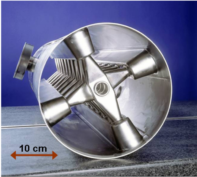
FIG. 1. (Color) Technical layout of the CH-prototype cavity (top), view into the superconducting CH cavity (bottom).
