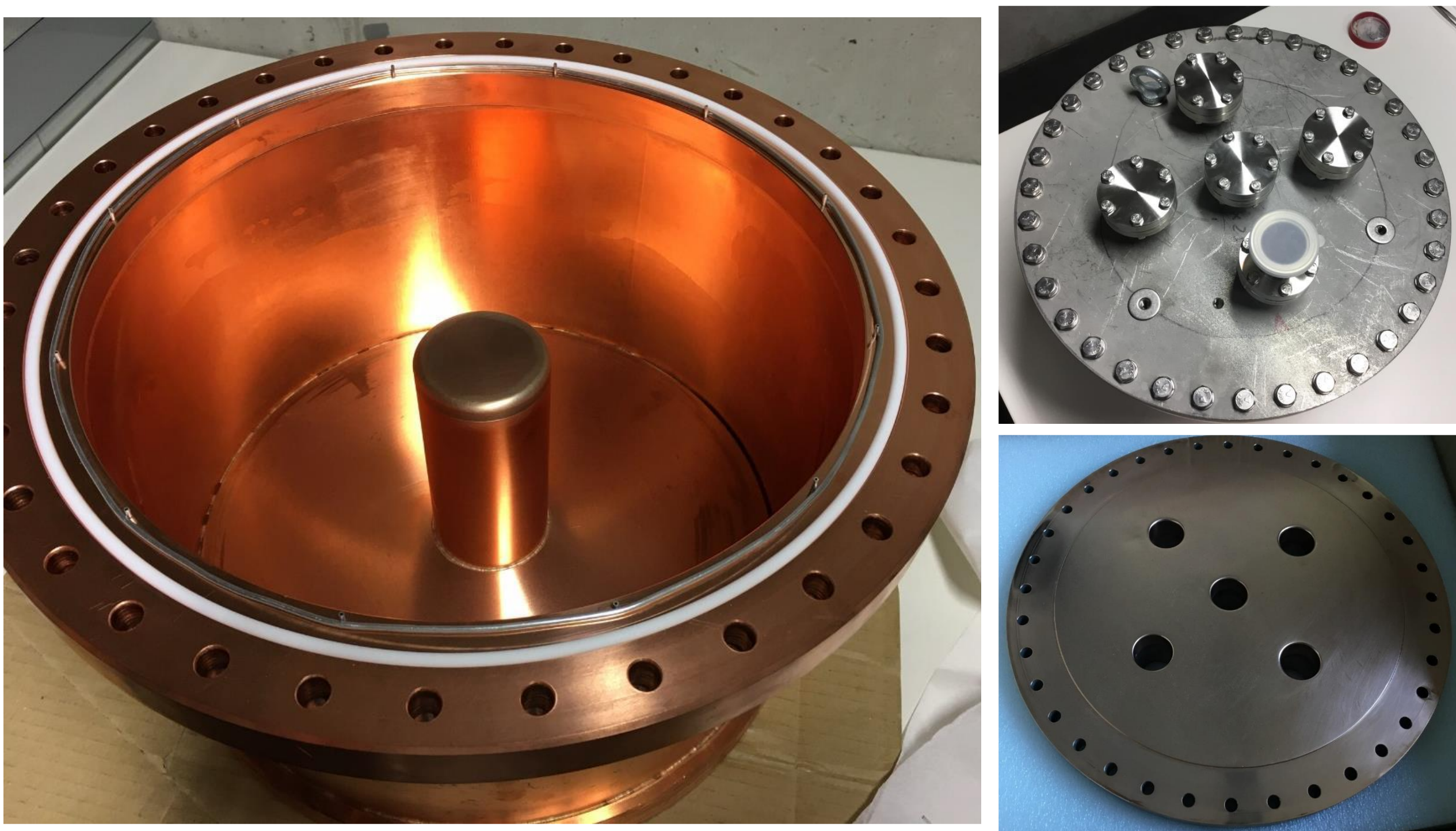
Figure 1: Structure of the shortest \lambda/4 coaxial cavity.
