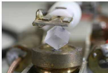
Figure 7.2: Photograph of a ZnGF single crystal mounted in the RUS set-up. The sample size is of \sim 5.351(2) \times 5.091(2) \times 4.252(2) \text{ mm}^2 .
