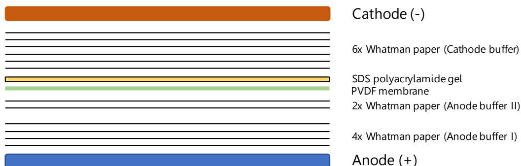
Figure 16 – Schematic representation of a semi-dry Western blot transfer system. In a semi-dry Western blot transfer system, the SDS polyacrylamide gel and the PVDF membrane are sandwiched between two stacks of Whatman paper and placed horizontally between two electrodes. The Whatman papers are soaked in the indicated buffers and the excess moisture and trapped air bubbles are removed during the assembling of the sandwich.
