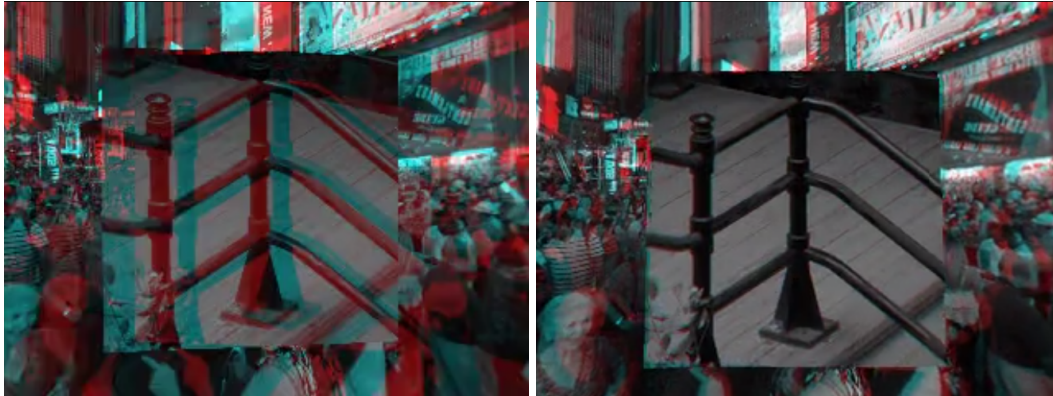
Fig. 5.3 Left / right anaglyph of the two eyes before (left) and after (right) a fixation movement. The images from the left and right eyes are converted to grey scale and then superimposed as two color channels of a single image.
