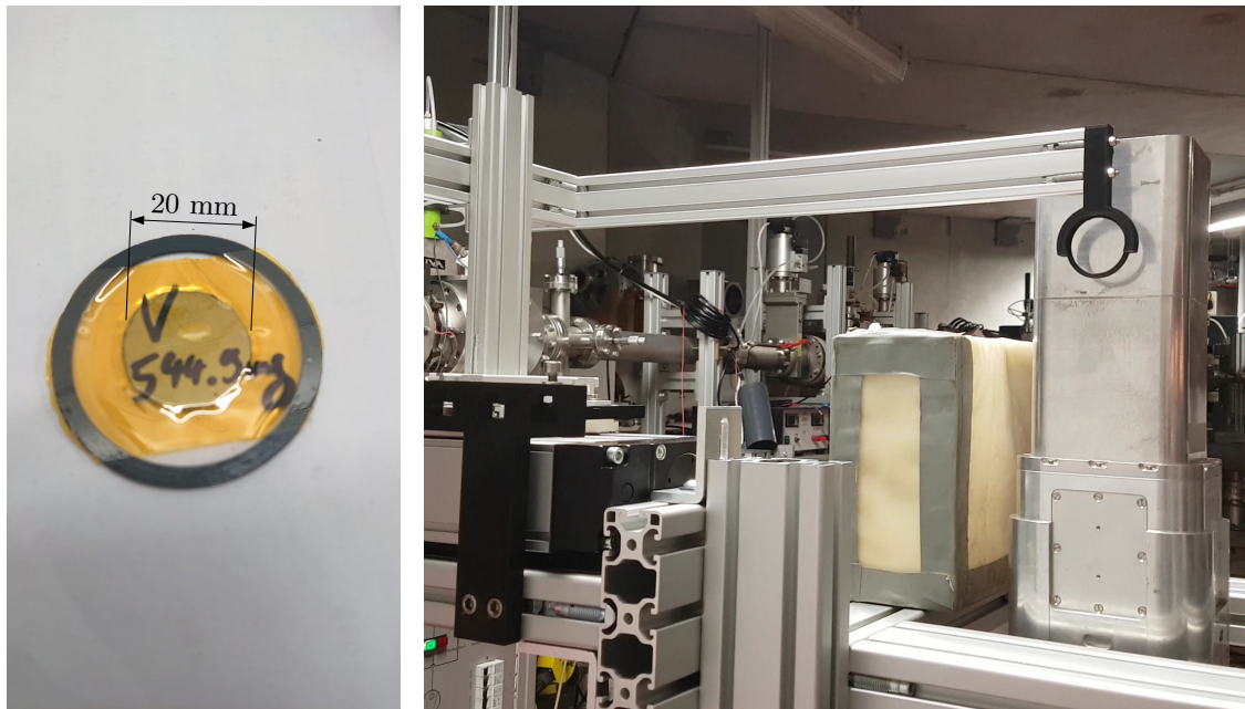
Figure 4.37: Sample preparation and fixation to the transport system. On the left side the ^{51}\text{V} sample is shown. The sample is kept in a central position by a polyimide foil glued to a ring of polymere. The picture on the right shows the sample transport system with an empty ring clipped to the sample holder in front of the clover detector.
