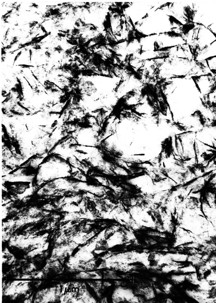
Fig. 5. Calcium-phosphate needles in a membrane section.
