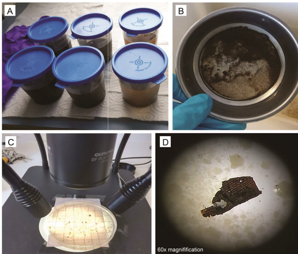
Figure 4.15 Short protocol exposition of charcoal extraction and identification. A) Samples dissolved in water and chlorinated; B) Wet-sieving; C) Quantification under microscope; D) Identification of charcoal morphologies.
