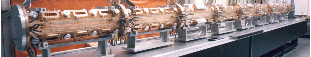
Fig. 3.1.3-2: The 8m-long LEDA-RFQ accelerator [YOU94].
