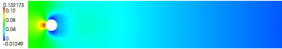
(a) Pressure (color) for the boundary fitted mesh in Fig. 9a.
