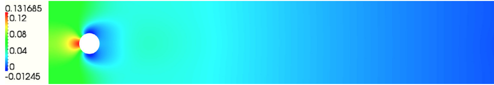
(b) Pressure (color) for the enriched scheme and the unfitted mesh in Fig. 9b.
