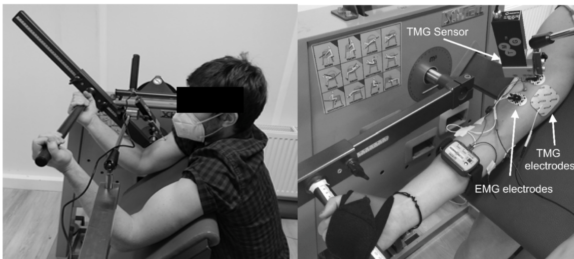
Fig. 2. Experimental set-up. Participants are seated in a biceps curling machine (left). The TMG sensor is placed on the m. biceps brachii and measures muscle belly displacement after an electrical stimulus. EMG records muscle activation during imagery conditions (right).
