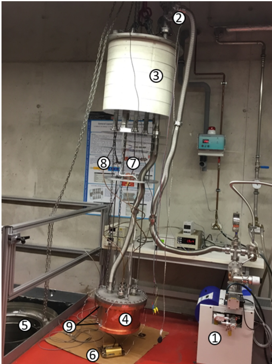
Figure 7.1: Photo of the prepared 340 MHz cavity, ready for installation in the cryostat: 1=turbo molecular pump station, 2=ion getter pump, 3=lid of the vertical cryostat, 4=cavity, 5=open cryostat, 6=heater, 7=coaxial cable for the input signal, 8=coaxial cable for the output signal, 9=temperature sensors.
