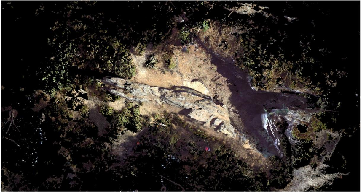
**Fig. 9a** *territorium metallorum* Tresminas/Jales, Gralheira ore vein: top view of Pos. 1. The two ore veins cross each other at an angle of about 40 degrees. In the middle of the picture the small rocky ledge as well as the channels and the Y-shaped cut of Pos. 1b adjoining it are visible (UAV photo: HCU Hamburg, M. Lindstaedt, K. Mechelke).
