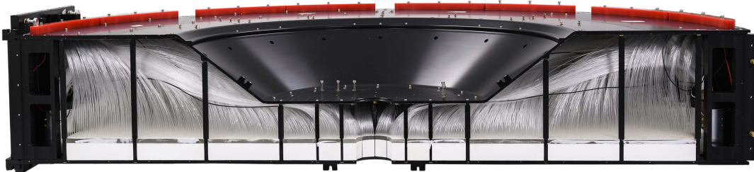
Figure 57: Photograph of one half of the FV0. The optical fibers connect the scintillators to the PMTs on the rim of the support structure, the black structure seen here. The center wall has been removed to show the scintillator, the surface matrix structure, and the optical fibers.
