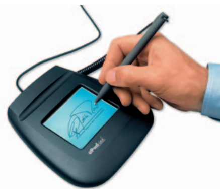
Figure 2: Capturing of Handwritten Signatures using a Pen Pad.
